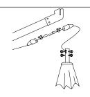
5. To assemble the lower and upper halves of the Umbrella Cable, locate the two ends of the Cable. Each of the (2) Cable ends has an oval Cable Protector attached. Place the (2) ends of the Cable Protector together and twist to screw the two halves together.
