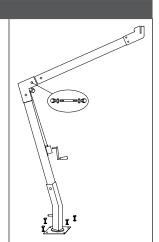
3. Using (2) persons, lift the Upper Pole and Lower Pole assembly to the vertical position. Place the square plate at the lower end of the Lower Pole on to the assembly of the Base Stand. Orient the Upper Pole with Upper Hook so that the Assembly is facing away from the Base Weights. Align holes of the square plate with the threaded holes on the Base Stand. Using the Hex Head Wrench, install (4) Hex Head Screws and (4) 1 1/4" Washers. Fully tighten.
